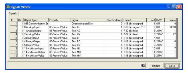
The signals viewer can be used although only one system is connected to the IntesisBox, *Modbus* or *BACnet*, and is very useful for supervision and test.
