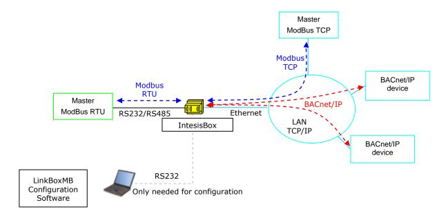
Integration of BACnet and Modbus using IntesisBox Modbus Server - BACnet/IP Client gateway
